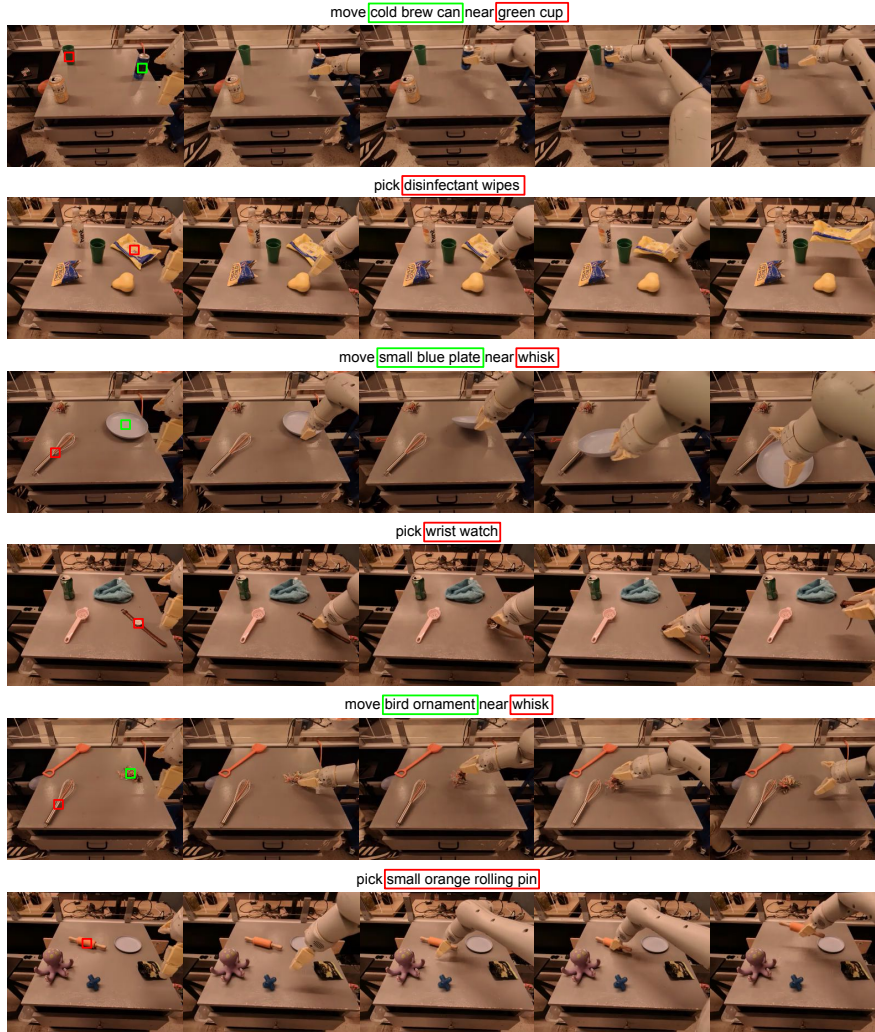
Figure 6: Example images of our policy detecting and grasping objects not seen during training time. The object detections are colored in correspondence to the text above the image, and the images are ordered left to right across time.
